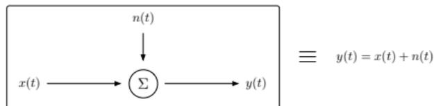
The noise  $n(t)$  is a 1 dimensional random signal Gaussian with zero mean, variance  $\sigma^2$  and probability distribution:
